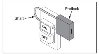
Figure 42. Switch disabled by a padlock.
